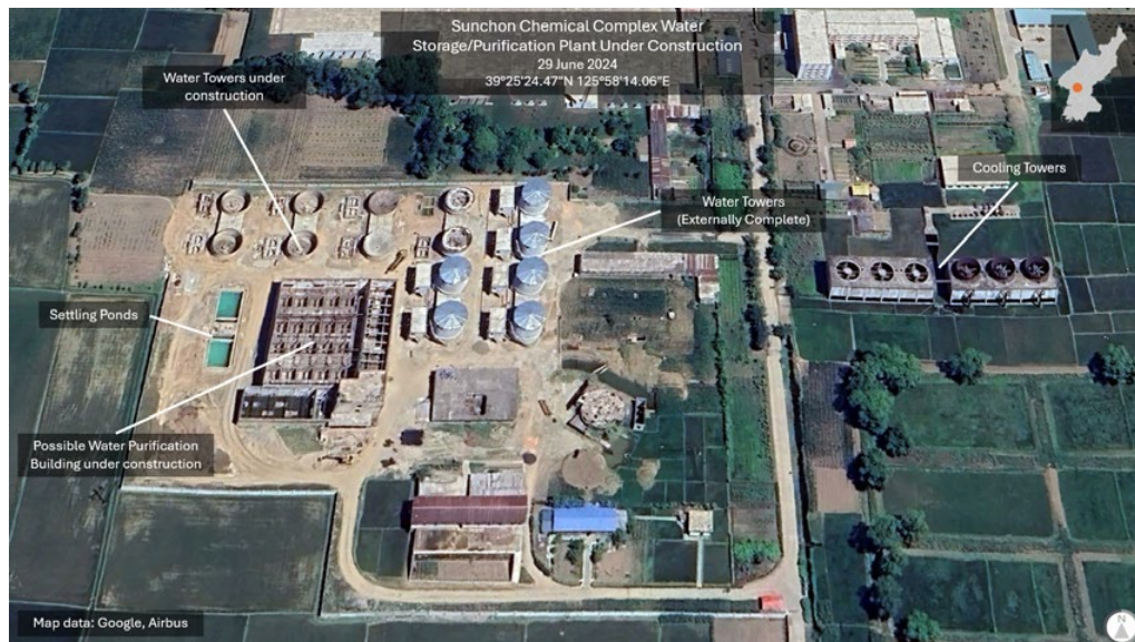
Figure 32: Probable water storage and purification plant for the Suncheon Chemical Complex and/or Pharmaceutical Factory
