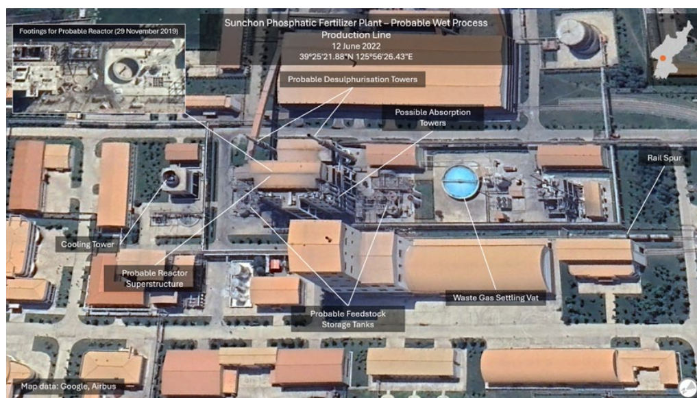
Figure 9: Probable wet process production area at the Sunchon Phosphatic Fertiliser Plant
