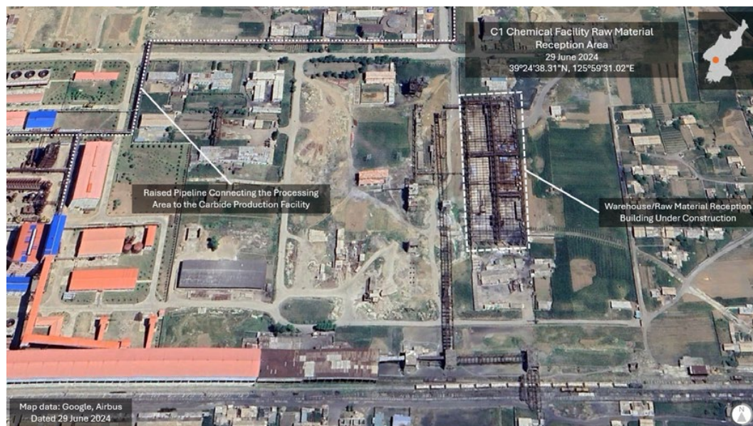
Figure 20: Raw material reception area at the C1 Chemical Facility
